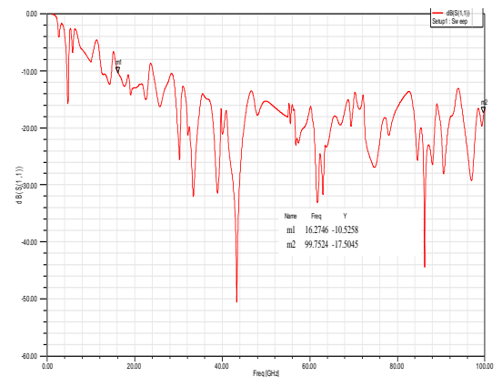
Figure.5. Return loss in frequency function of the proposed printed-IFA with Interconnected CRLH unit cell
